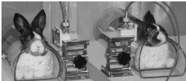
Fig. 3. Experimental setup for microwave exposure.
