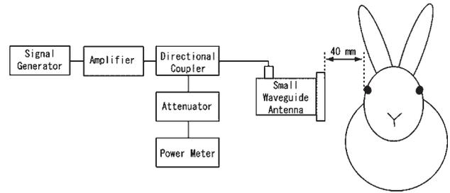
Fig. 1. Diagrammatic representation of the animal exposure system.
