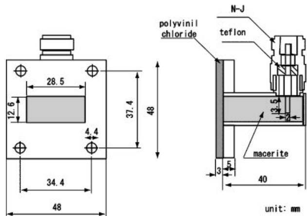
Fig. 2. A schema of a dielectric-loaded small waveguide antenna.
