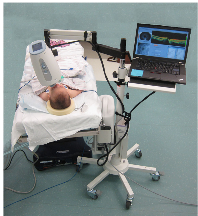
Fig. 1 Optovue iVue optical coherence tomography unit, in use performing retinal imaging on an infant under sedation prior to cranial vault expansion
