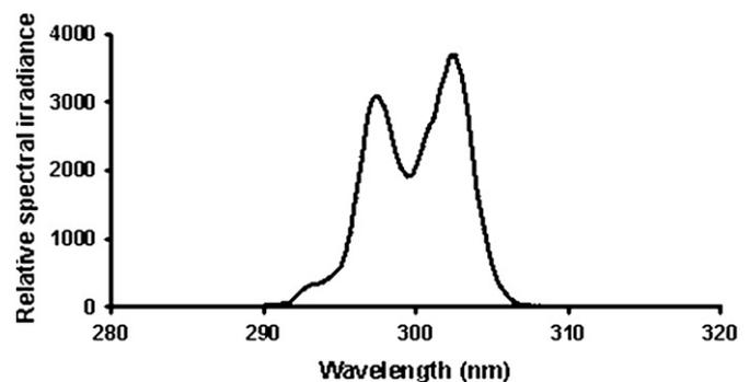
**Fig. 2.** Spectral irradiance of UVR in the exposure plane.
